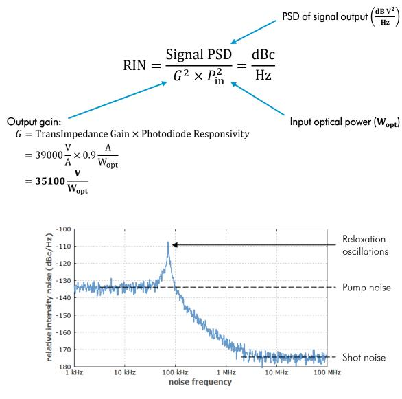
Simulated RIN of a 1064-nm Nd:YAG laser with 100 mW average output power. Source: https://www.rp-photonics.com/relative\_intensity\_noise.html
