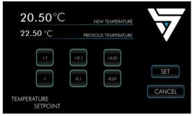
**IMPORTANT:** The value of the setpoint is saved in the internal memory of the system and recalled when the device is restarted.
